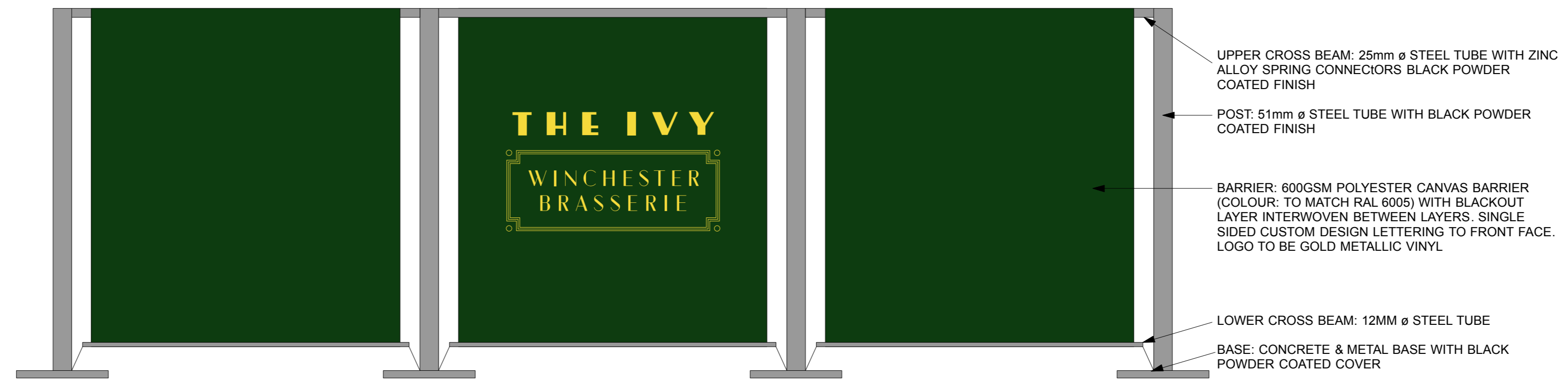
5 EXTERNAL BARRIER - ELEVATION 1:10 @ A1 / 1:20 @ A3
