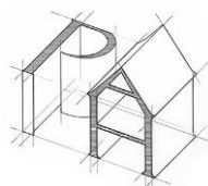
Fig 27 – principal areas affected by bird perching and roosting.
