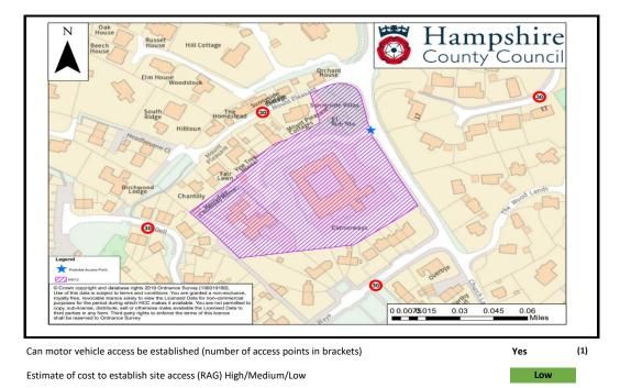
The options for this site include utilising the existing access (low-cost option) or potentially relocating the access further south on Church Lane to improve visibility splays (medium cost). There is also the potential to improve the pedestrian and cycle access from the site down the existing track located to southwest of site which links to Willis Waye.
