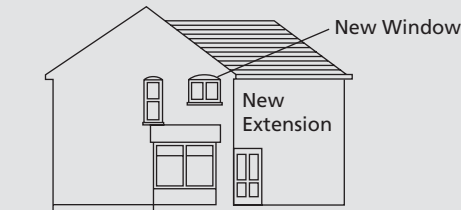
2 SIDE ELEVATION (NORTH)
