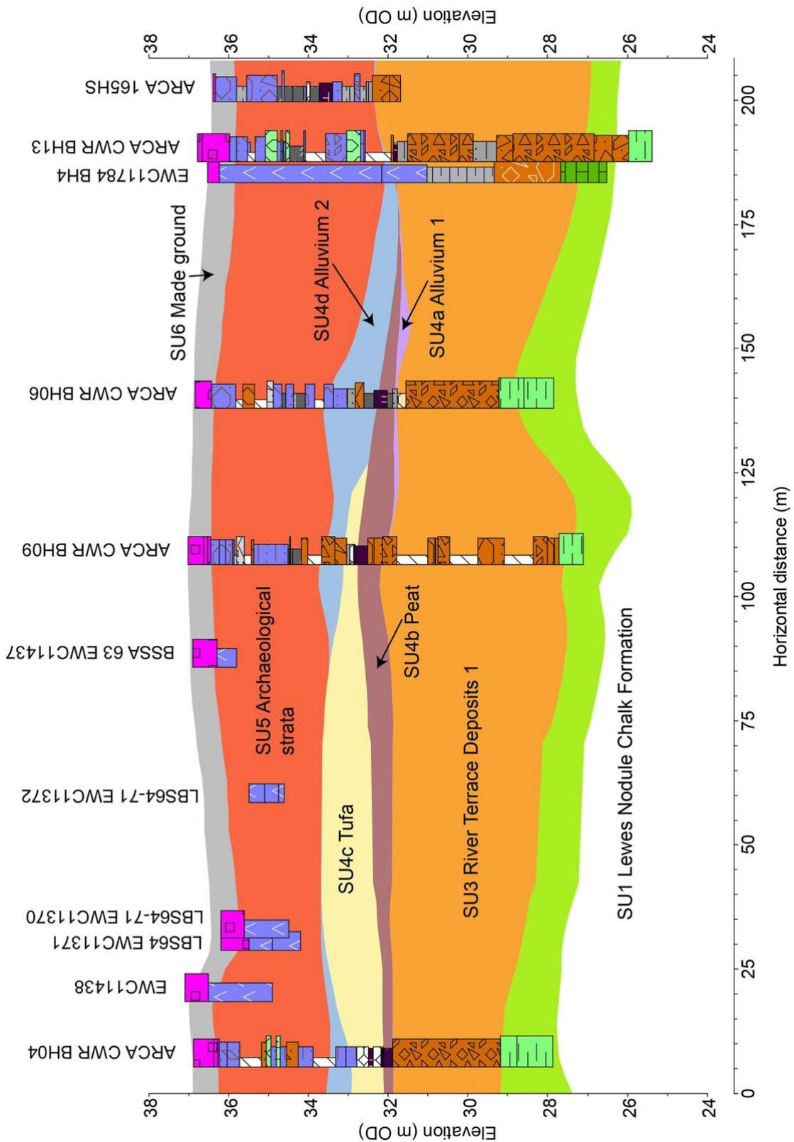
Figure 15. North to south composite cross section through the CWR site on the basis of ARCA CWR boreholes and other records in the ARCA stratigraphic database
