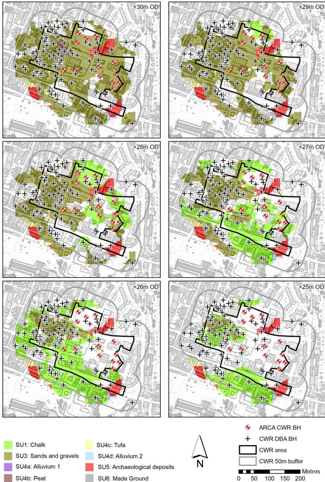
Figure 17. Modelled distribution of stratigraphic units at 1m depth slices (7–12m bgl)
