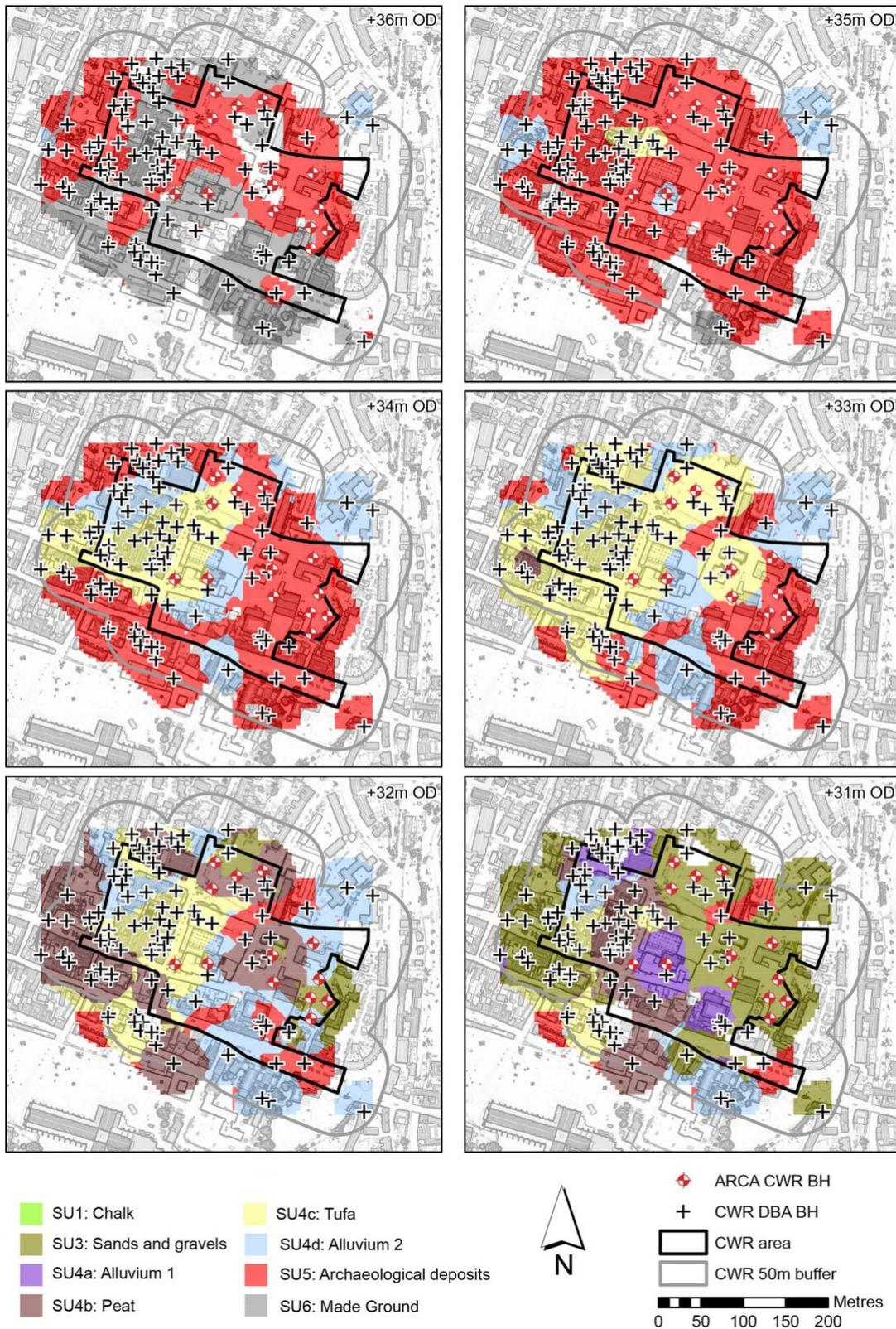
Figure 16. Modelled distribution of stratigraphic units at 1m depth slices (1–6m bgl)
