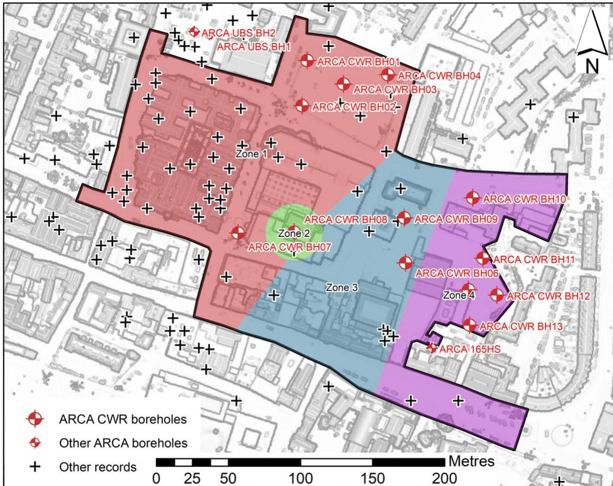
Figure 21. Zonation of the CWR on the basis of stratigraphic characteristics
