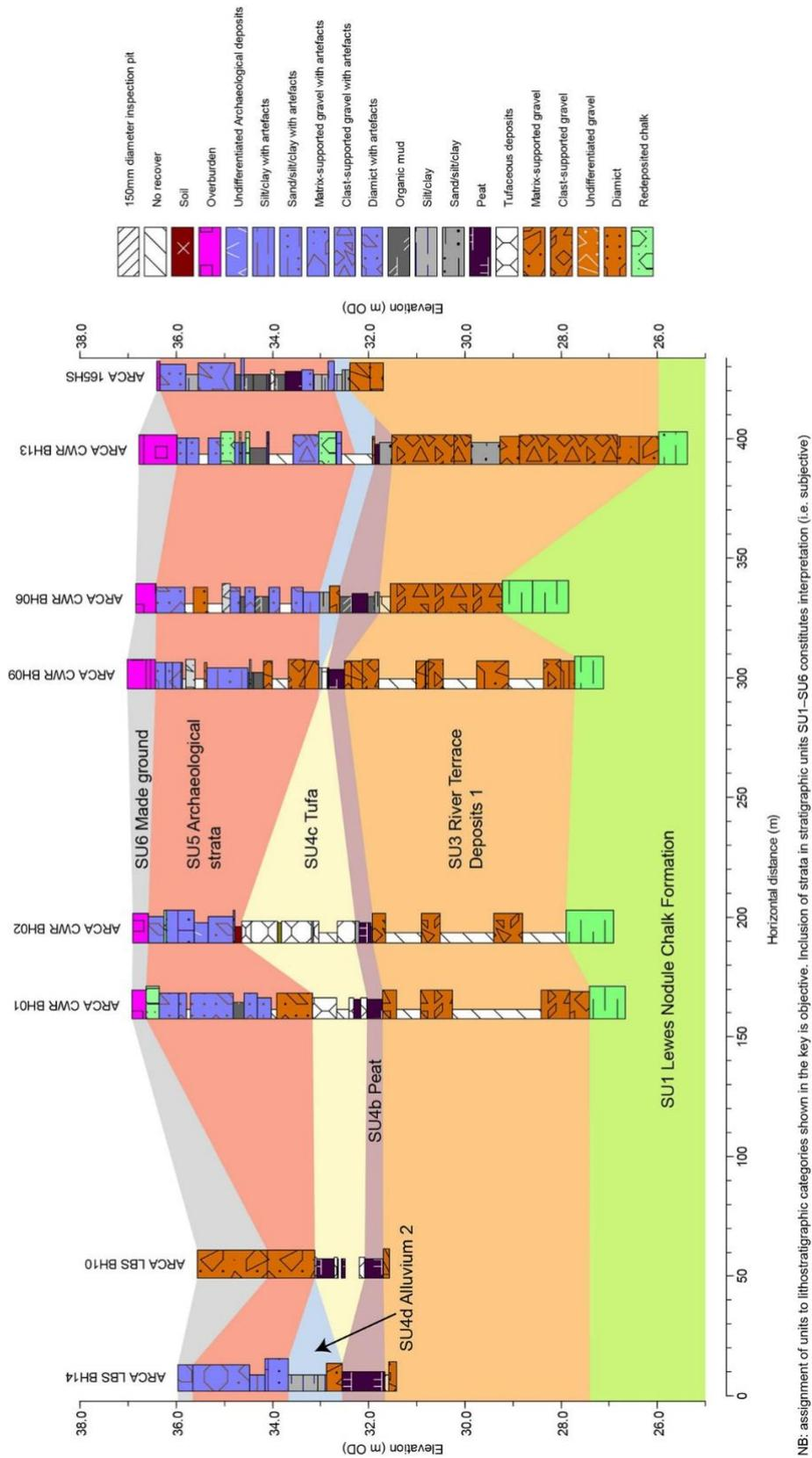
Figure 5. North–south composite cross section through ARCA’s CWR, Lower Brook Street (LBS) and 165 High Street boreholes
