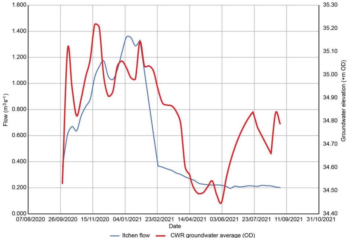
Figure 8. Average groundwater in the CWR study area plotted against flow in the River Itchen as measured at the Seward's Bridge monitoring station, Alresford
