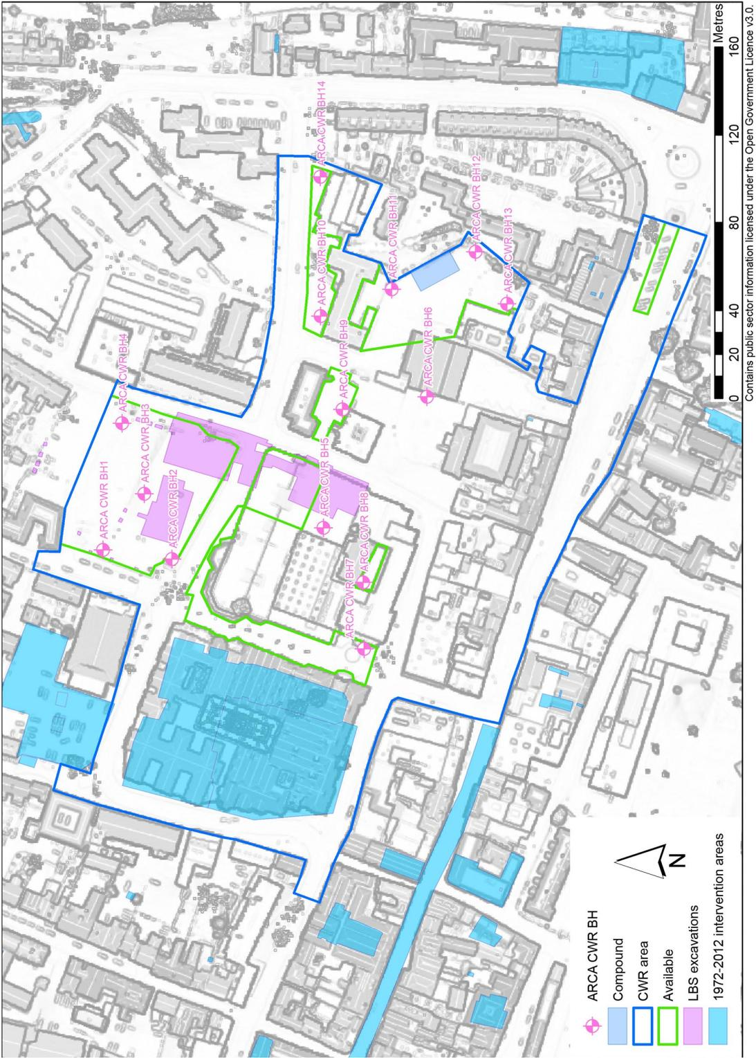
Figure 7. Proposed test pit and borehole locations
