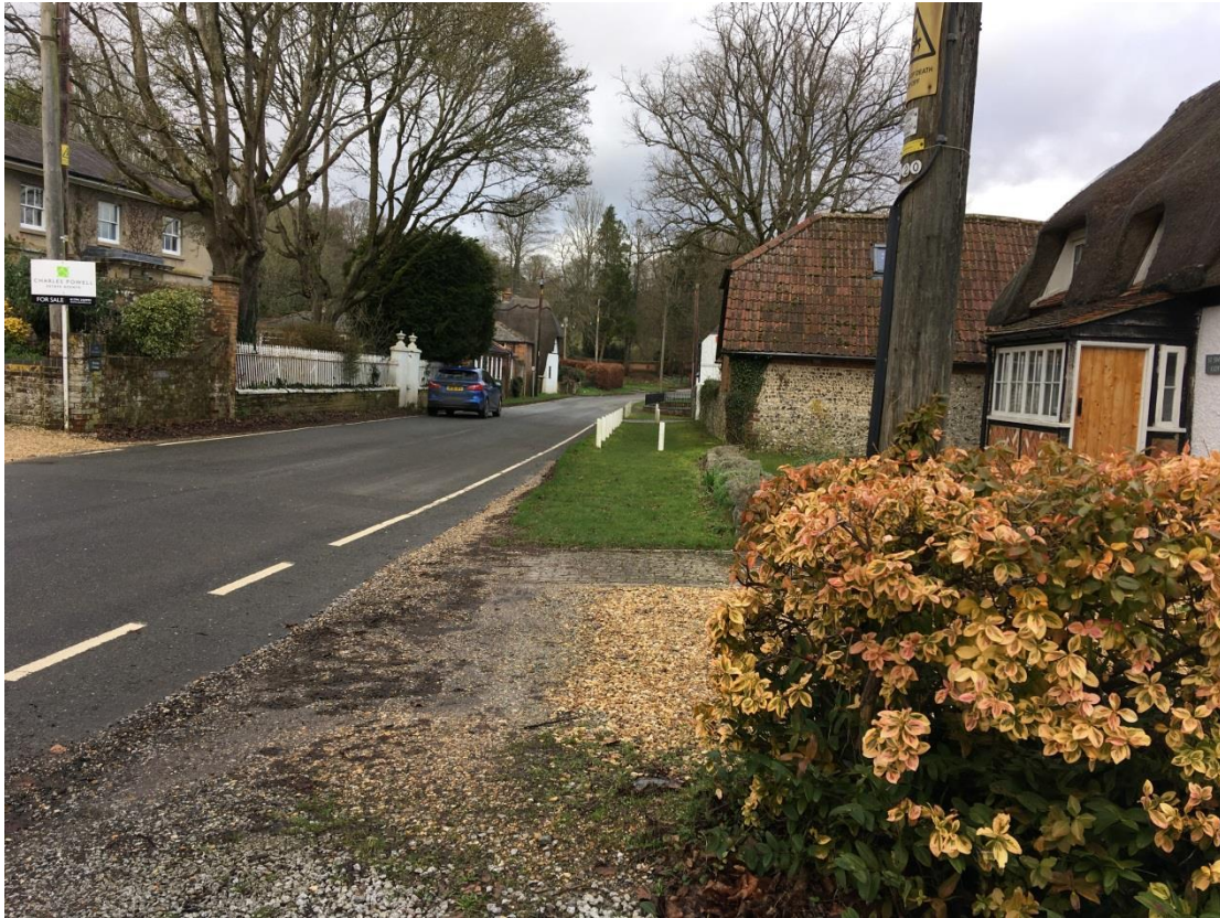
Photograph 3 – Visibility at the Site Access looking to the right from 2.4m 'x' distance
