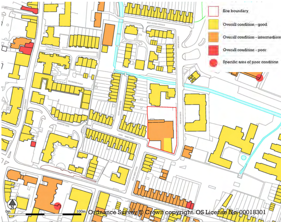
Figure18: External building condition
