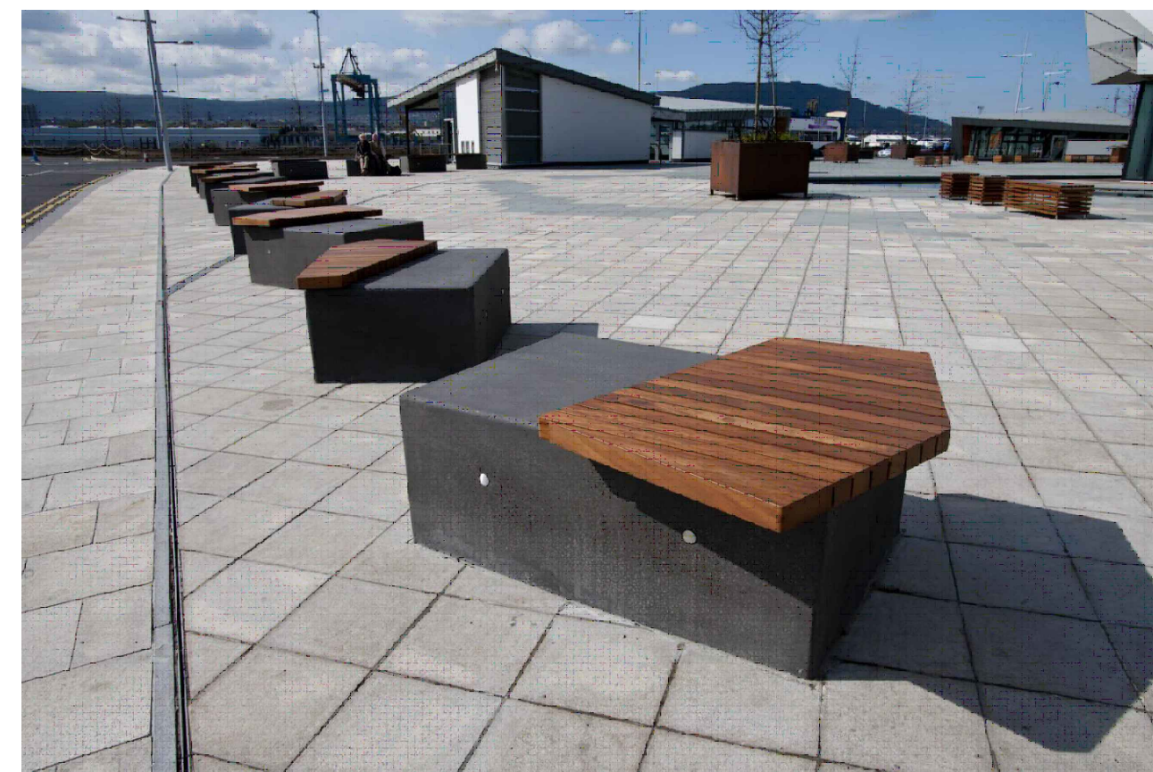
Townscape PAS 68 Blocks with Banyan seat tops (Sapele timber tops)
